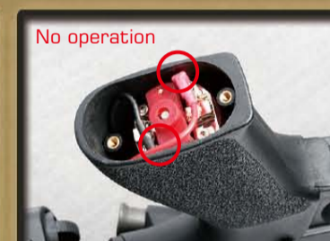
Check the wire set contact with motor.
