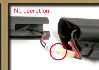
Check the battery and connector.
