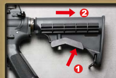
Press the stock release lever to unlock.
