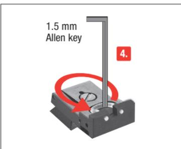
4. Slightly loosen the headless screw and place the sight in the dovetail guide.
