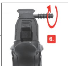
6. Push down the slide catch lever (release the slide).
