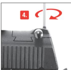
4. Using a 1.5 mm Allen key, to fix the slide racker.
