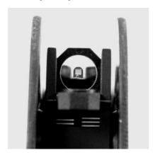
Flip down the two ringsight slide flaps and lift up the slide located on the front face of the frontsight support. It is necessary to align the target, the green luminescent spot (materialising the support), and the two red luminescent spots which appear on the sighting rule support for direct grenade firing when this sighting rule is folded back.
